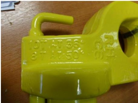
The photo shows a RH lug with the loading clearly marked for spreader beam use.
