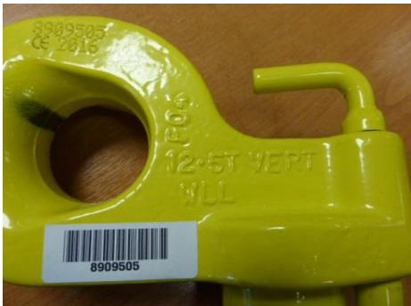
The reverse of the lug has the loading for lifting frame use.
